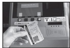
Fare boxes on board CTtransit local, express, and CTfastrak buses issue 2-Hour Passes (transfers) and All-Day passes using bar-code reading technology rather than magnetically encoded stripe technology. The bar code is printed on the front of the pass. Scan the bar code on the window with the red light on the fare box – a tone will sound indicating acceptance.
